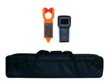
ES1001 high/low voltage current meter lock clamp is a high voltage measuring device consisting of a special current meter clamp and an insulating rod. The current measuring clamp is attached to an insulating rod for current measurement on insulated cables with a maximum of 60kV or on bare cables of maximum 35kV. Without the insulating rod, the clamp can also be used as a high-precision lowvoltage current meter clamp or leakage current meter, capable of measuring (leakage) currents down to 0.1mA.
