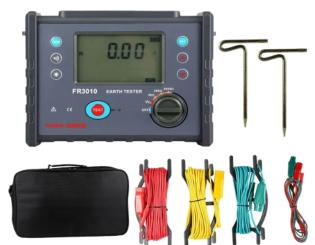
Model FRS3010 digital earth resistance meter uses three-wire voltage-current method for measuring earth resistance, while it performs low-resistance measurement using two-wire method. The large backlit LCD display, the microprocessor structure and the adjustable alarm threshold ensure convenient handling, stable operation and high accuracy.
