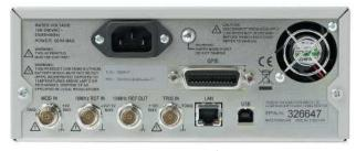
Rear panel mounts the digital interfaces and the rear I/O connectors. (Note: GPIB interface is an option)
